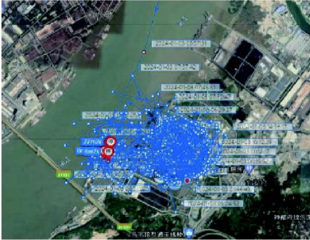
[Figure 3: AIS Trajectory Change When UAV Countermeasure Equipment Was Transmitting]
